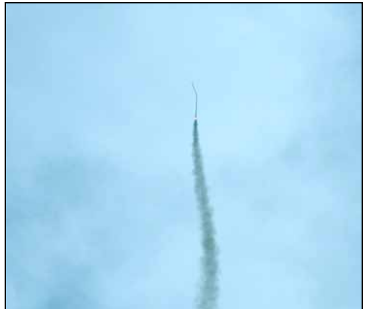
Figure 2: Too much flexing can cause the tubes to buckle and the rocket to fail.
